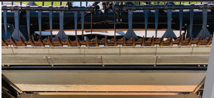
Code: S58 OEM Code: MACDON 102336 STAINLESS STEEL 3MM BOLT ON LEFT HAND SKID PLATE SUIT MACDON 973-974
